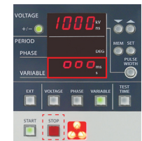
Continuous testing with 000 setting until the STOP switch is pressed.
